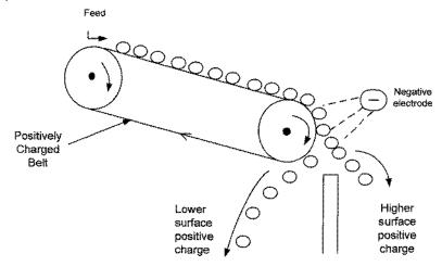
Fig. 1.4 Principle of electrostatic cleaning.
