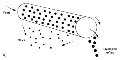
Fig. 1.2 Screen geometries: (a) rotary screen, (b) principle of flatbed screen.
