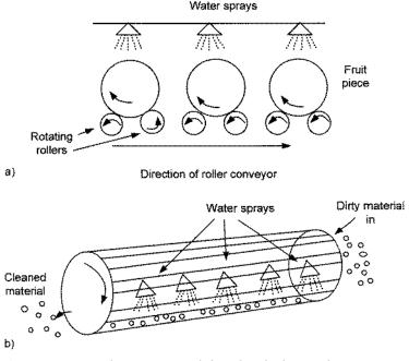
Fig. 1.5 Water spray cleaning: (a) spray belt washer, (b) drum washer.
