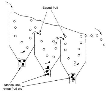
Fig. 1.6 Principle of flotation washing.
