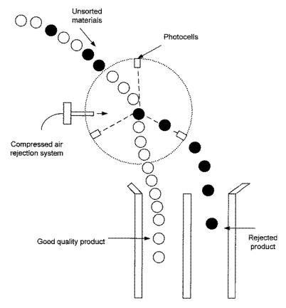
Fig. 1.9 Principle of colour sorter.
