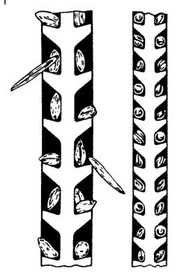
Fig. 1.8 Cross-section of disc separators for cleaning cereals.
