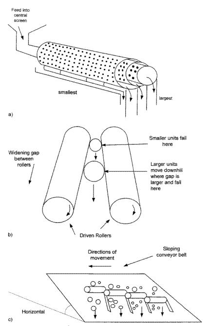
Fig. 1.7 Some geometries of size sorting equipment:
