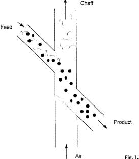
Fig. 1.3 Principle of aspiration cleaning.
